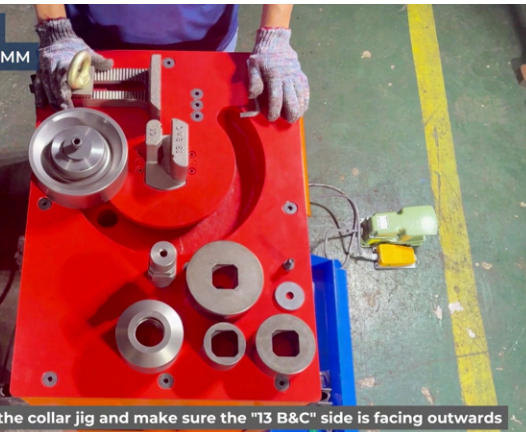
COMBINATION #1.1 FOR REBAR DIAMETER 13MM COLLAR JIG "13" SIDE
